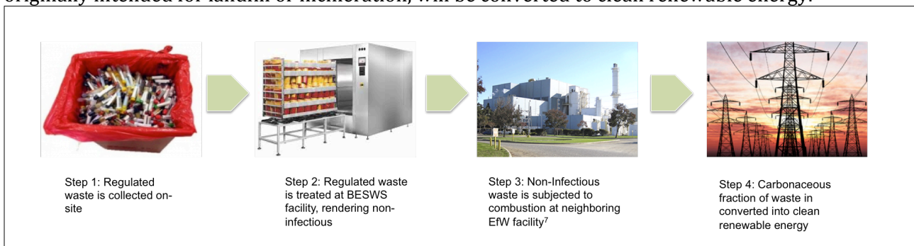
Figure 1. Flowchart of BESWS implementation of Waste to Energy processes. Regulated waste originally intended for landfill or incineration, will be converted to clean renewable energy.
